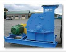
The Rocktec HSI Bath impactor is specifically designed to crush waste Alumina bath which can then be recycled and used in the Aluminum production process. A high reduction ratio is achieved by Tungsten tipped flails and Tungsten tipped anvils, these are set to determine the finished product size. The internal ledges combined with Tungsten tips/anvils provide high efficiency and durability.
