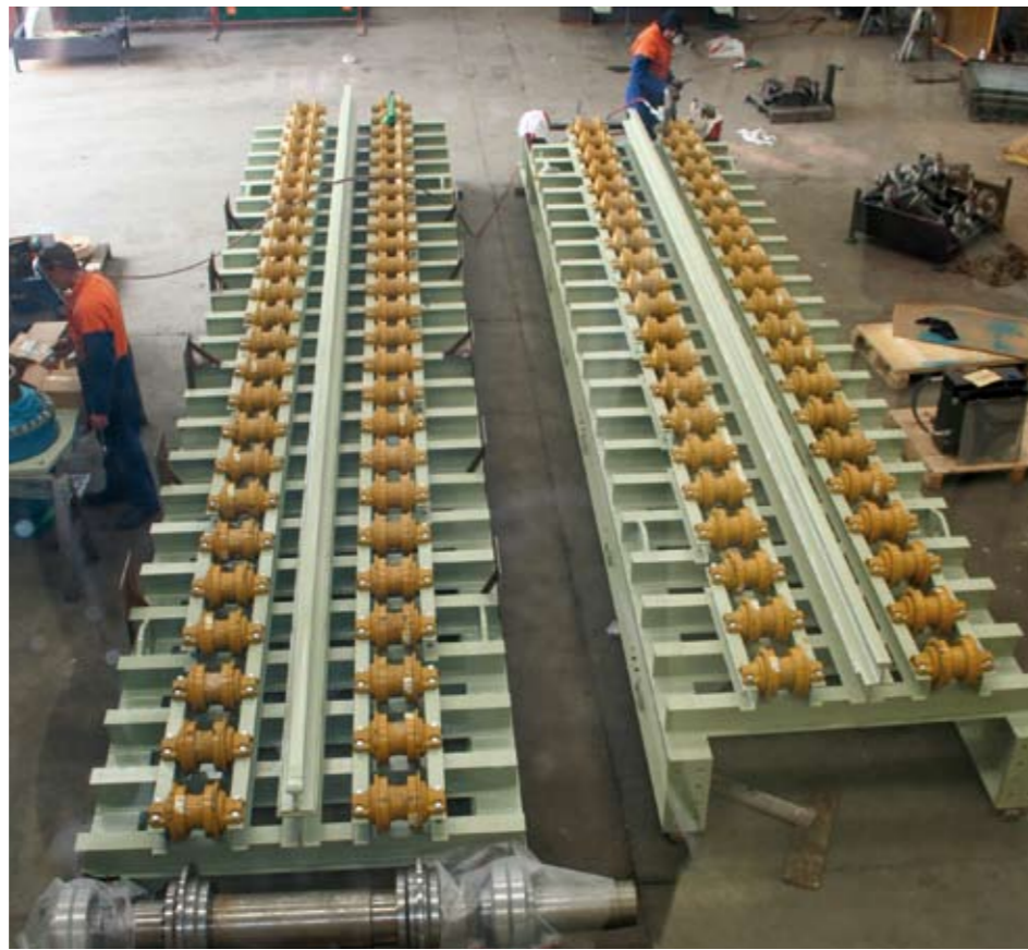
Manufacture of Apron Feeders for BHP mine site, Western Australia
