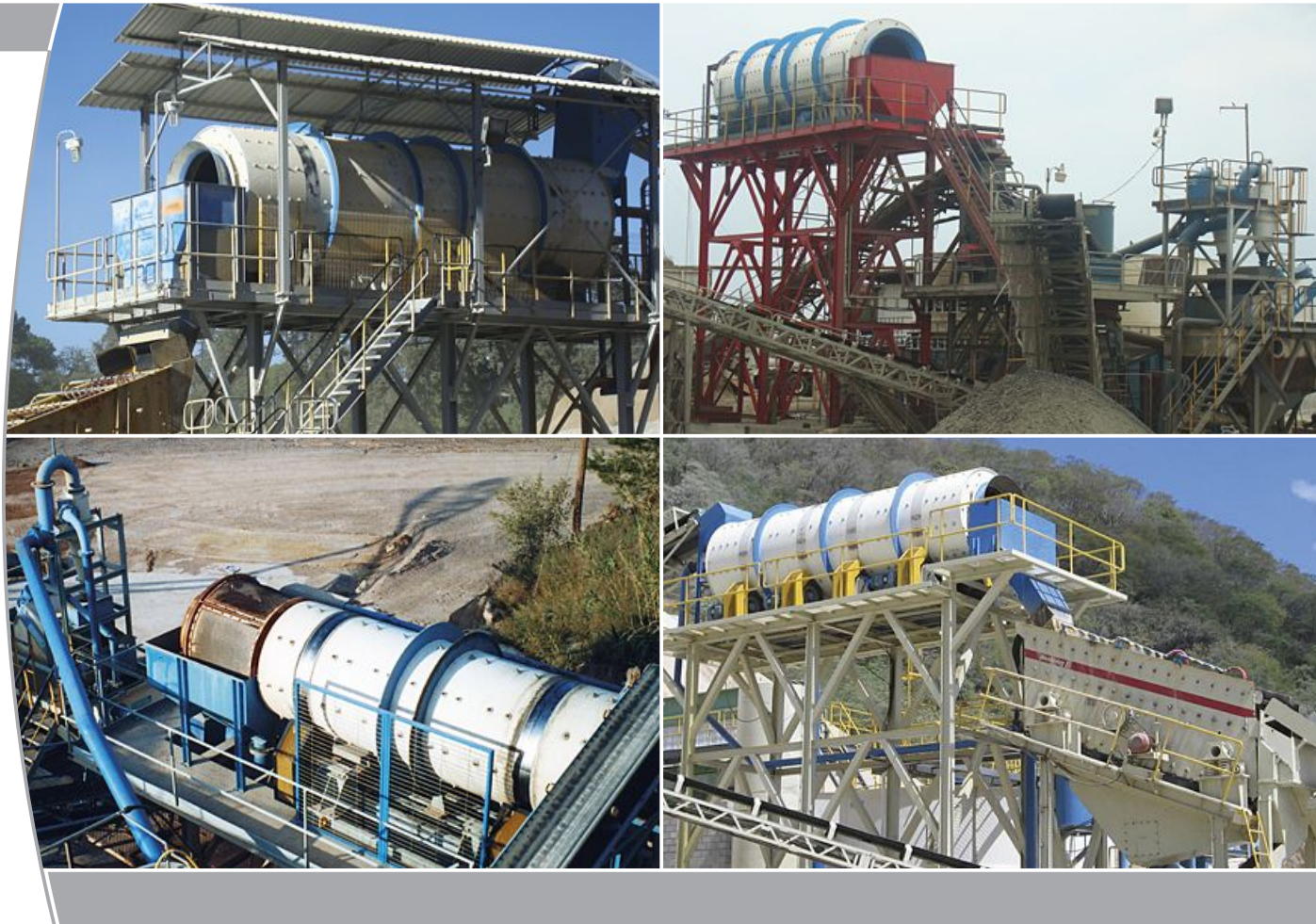
Type CM 18.05 for kaolin/silica sand treatment
