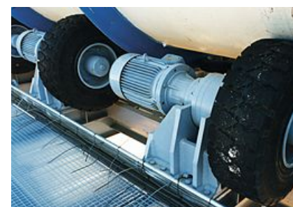
Drive system by motor reducers
