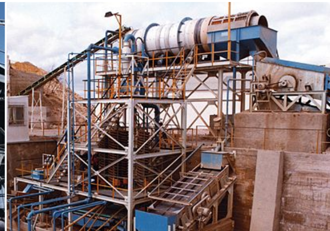
Type CM 20.06 for tin ore washing
