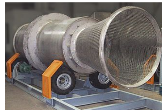
Type CM 16.04 in stainless steel construction
