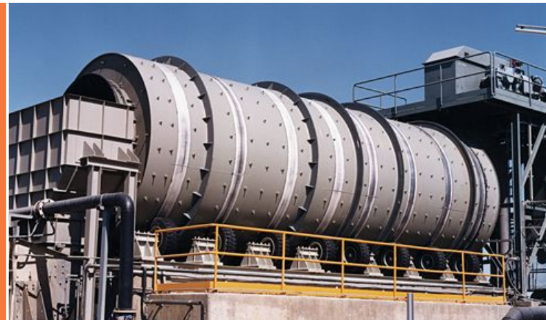
Type CM 37.11 for uranium ore washing
