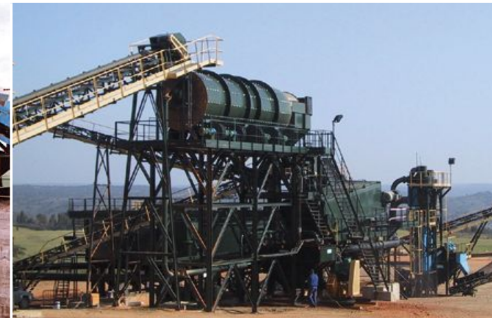
Type CM 25.08 for sand & aggregates washing
