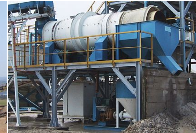
Type CM 14.04 for silica sand washing
