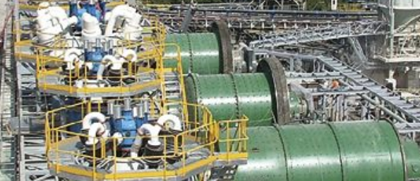
Grinding and classification circuit tailings (copper)
