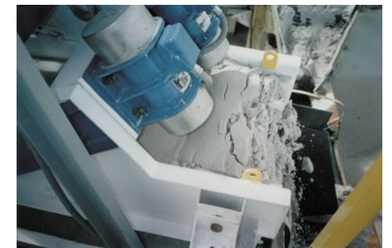
Mortar sand dewatering
